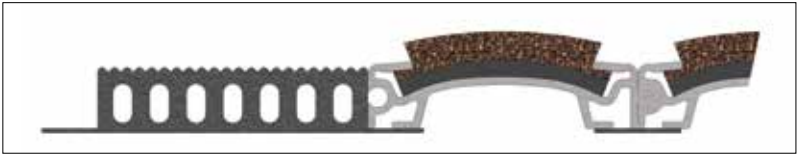
Rubber fill in profiles ensure a neat matwell finish and facilitate cutting on site
